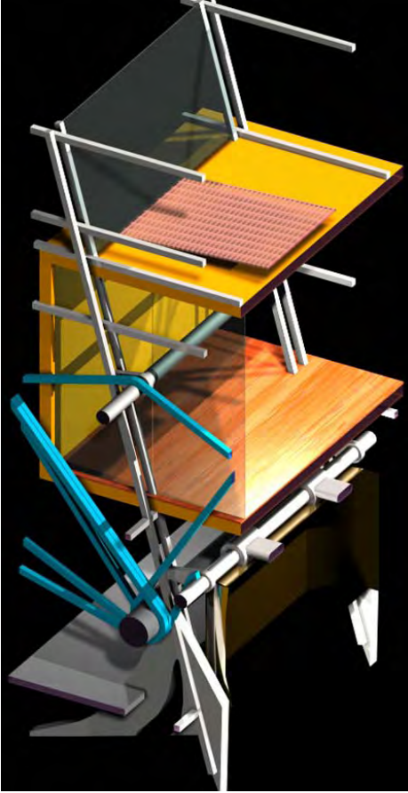
Figure 23: Digital Wall Section, by Ramirez.
