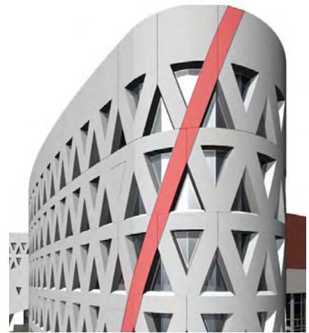
Figure 9: Perspective of the precast computer model illustrating the compound helical geometry.
