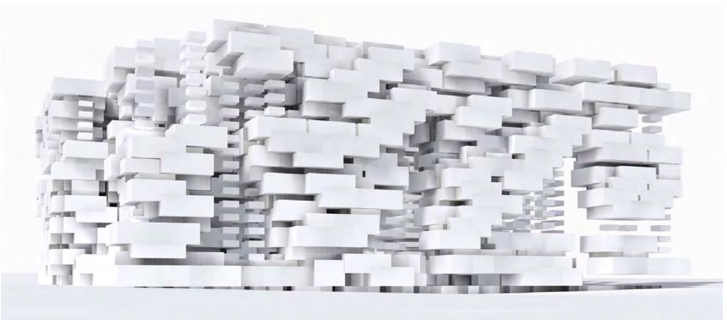
Figure 1. A housing arrangement for 200 units is constructed using a scripted algorithm based on cellular automata theory. While the final form of the arrangement was unpredictable, the programmatic requirements were predicted to be satisfied
