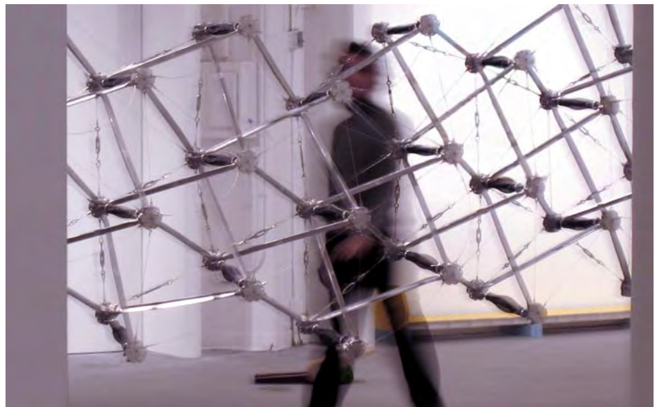
A full-scale prototype of an actuated tensegrity structure for use within a responsive building envelope. This prototype was built from cast aluminum pieces that were first rapid prototyped from form·Z models. The structure is programmable and responsive to its surrounding environment. In the photograph above the structure is not yet clad.
